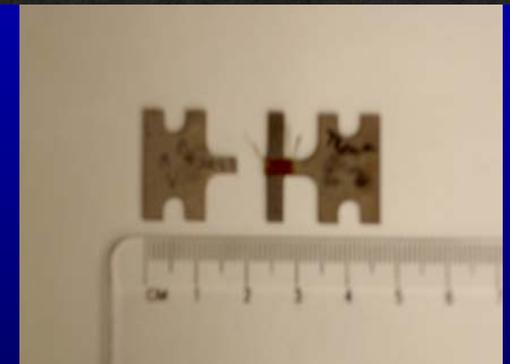
A specially-designed specimen was used along with an Ernest Fullam Tensile Stage to perform creep experiments at temperatures up to 760°C and loads up to 1000lbs. EBSD orientation maps can be performed both before and after creep deformation as well as *during* the creep deformation experiment.
